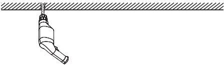
1. Drill a \varnothing 6\text{mm} hole
